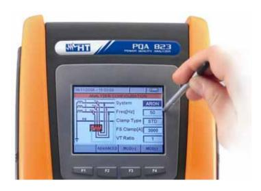
A wide (320x240pxls) graphical color TFT display with "touch screen" it's available for each model in order to access to any internal function by using the supplied pointer pen
